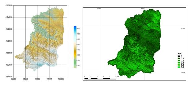
Figure 5. DEM and NDVI maps incorporated in the application.
