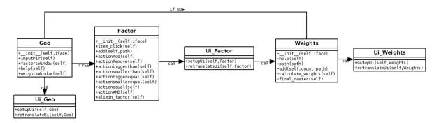
Figure 6. GeoDecision class diagram.
